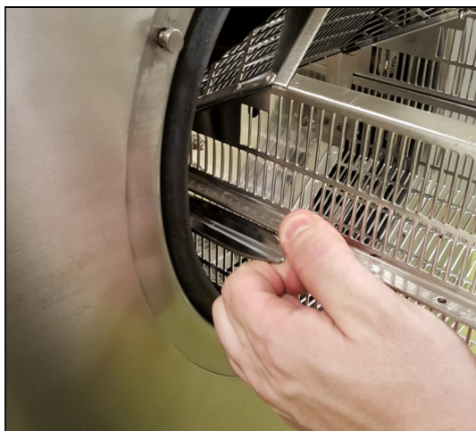
Figure 20 - Lock mechanism (the middle of the picture) which is pressed up to release the food basket container; right and left side of the basket
