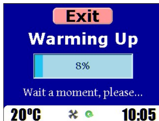
Figure 9 - Autoheat mode, the heating elements are activated, the fan is spinning
