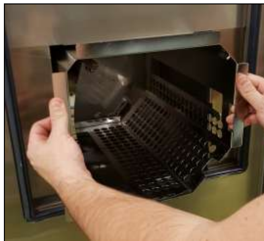
Figure 26 - Air duct plate pulled halfway out
