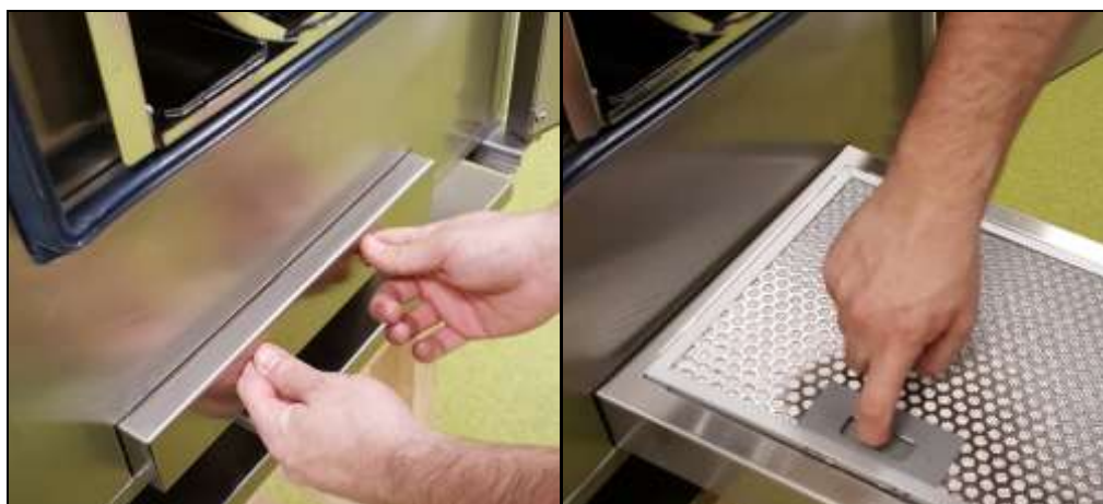
Figure 35 - Air filter partially pulled out
