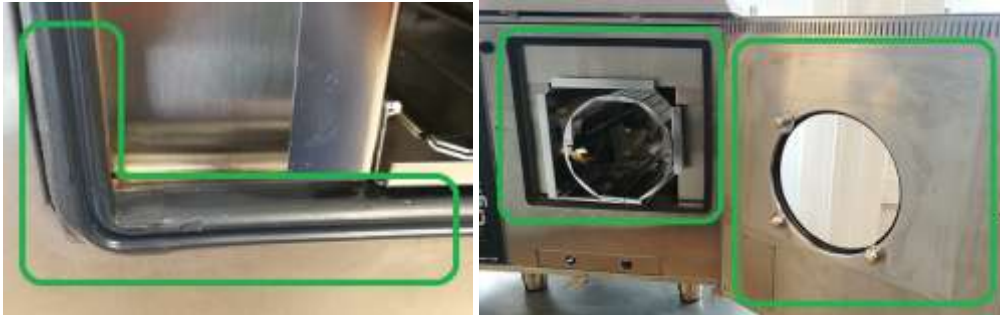
Figure 28 – Clean any residues, food particles or grease, on the door seal gasket as well as the inside door panel.
