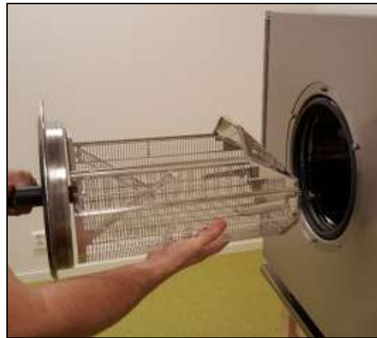
Figure 22 – Pull out food basket container completely.
