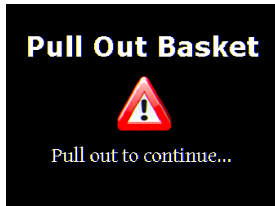
Figure 17 – The machine chirps approx. 10 seconds before it is time to pull out the basket, and the cook is ready.
