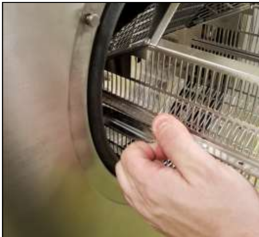
Figure 21 - Lock mechanism (the middle of the picture) which is pressed up to release the food basket container; right and left side of the basket
